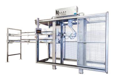
Predominantly know for our automatic bagging equipment, we recently introduced the industry's first-known robotic top pad inserter. The six-axis robot places cardboard top pads in different-sized produce boxes. As boxes move down a conveyor, the robotic system determines the box size and picks the appropriate pad for each box.
