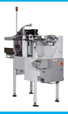
The SAS Automatic Pouch Bagger is the most reliable, consistent pouch bagging machine in the apple market. This workhorse will increase your bags per minute and dramatically reduce your labor costs. We utilize servo controls for precise and accurate bag filling and handling. The ultra soft fill lift will handle all varieties of apples in 2lb - 6lbs.
